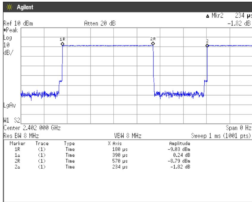
$$\text{Duty Cycle} = \text{Ton} / (\text{Ton} + \text{Toff}) = 390[\mu\text{s}] / (390[\mu\text{s}] + 234[\mu\text{s}]) = 62.50[\%]$$
