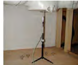
Figure 11.1 Dipole Verification Test Setup Diagram & Photo
