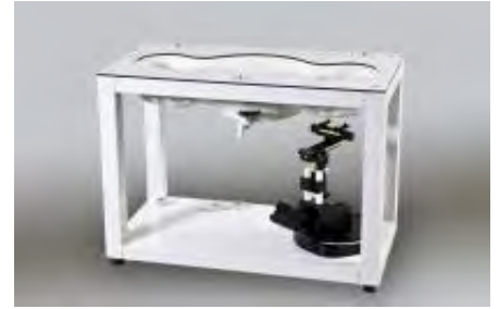
Figure 3.6 SAM Twin Phantom
