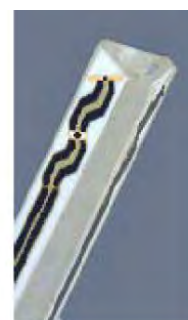
Figure 3.3 Probe Thick-Film Technique
