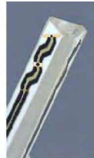
Figure E.2.2 Probe Thick-Film Technique
