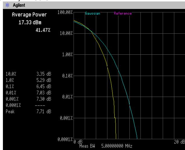
**64QAM, BW 15MHz, RB75-0**
