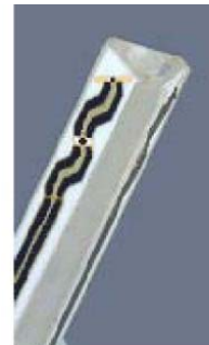
Figure E.2.2 Probe Thick-Film Technique
