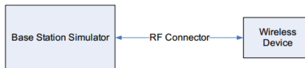
Figure 9.1 Power Measurement Setup
