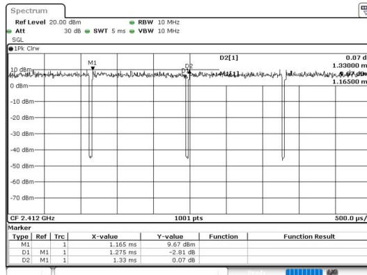
$$\text{Duty Cycle} = \text{Ton} / (\text{Ton} + \text{Toff}) = 1275[\mu\text{s}] / (1275[\mu\text{s}] + 55[\mu\text{s}]) = 95.86[\%]$$
