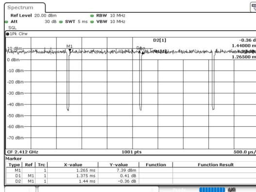
$$\text{Duty Cycle} = \text{Ton} / (\text{Ton} + \text{Toff}) = 1375[\mu\text{s}] / (1375[\mu\text{s}] + 65[\mu\text{s}]) = 95.49[\%]$$
