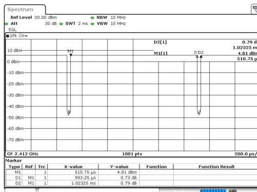
$$\text{Duty Cycle} = \text{Ton} / (\text{Ton} + \text{Toff}) = 993.25[\mu\text{s}] / (993.25[\mu\text{s}] + 30[\mu\text{s}]) = 97.07[\%]$$
