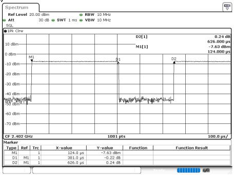
Duty Cycle = Ton / (Ton + Toff) =  $381[\mu s] / (381[\mu s] + 245[\mu s]) = 60.86[\%]$
