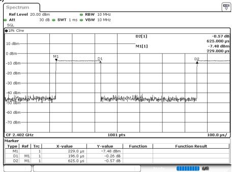
Duty Cycle = Ton / (Ton + Toff) =  $196[\mu s] / (196[\mu s] + 429[\mu s]) = 31.36[\%]$
