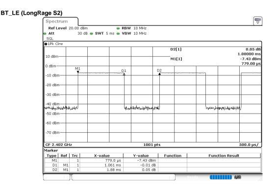
Duty Cycle = Ton / (Ton + Toff) =  $1061[\mu s] / (1061[\mu s] + 819[\mu s]) = 56.44[\%]$
