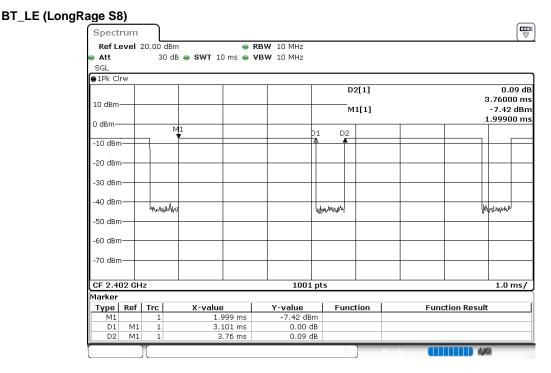
Duty Cycle = Ton / (Ton + Toff) =  $3101[\mu s]$  / ( $3101[\mu s]$  +  $659[\mu s]$ ) = 82.47[%]
