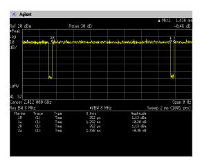
Duty Cycle = Ton / (Ton + Toff) =  $1392[\mu s]$  / ( $1392[\mu s]$  +  $44[\mu s]$ ) = 96.94[%]
