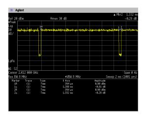
Duty Cycle = Ton / (Ton + Toff) =  $1288[\mu s]$  / ( $1288[\mu s]$  +  $44[\mu s]$ ) = 96.7[%]
