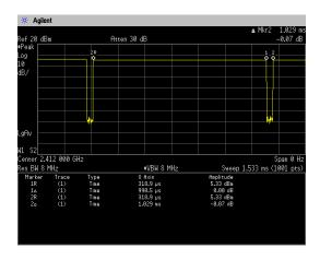
Duty Cycle = Ton / (Ton + Toff) =  $990.5[\mu s]$  / ( $990.5[\mu s]$  +  $38.5[\mu s]$ ) = 96.26[%]
