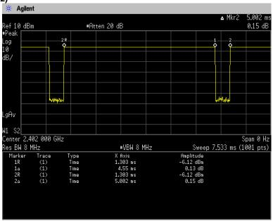
Duty Cycle = Ton / (Ton + Toff) =  $4550[\mu s] / (4550[\mu s] + 452[\mu s]) = 90.96[\%]$
