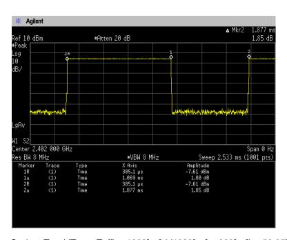
Duty Cycle = Ton / (Ton + Toff) =  $1069[\mu s] / (1069[\mu s] + 808[\mu s]) = 56.95[\%]$
