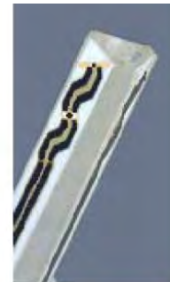
Figure E.2.2 Probe Thick-Film Technique
