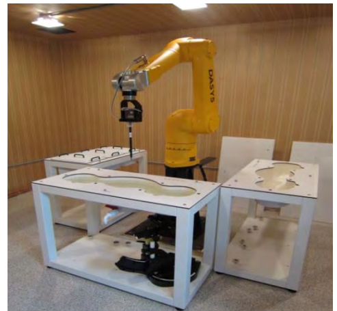
Figure E.7.1 DASY5 Test System
