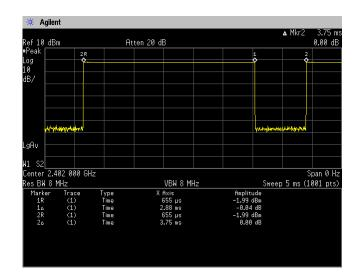
Duty Cycle = Ton / (Ton + Toff) =  $2880[\mu s] / (2880[\mu s] + 870[\mu s]) = 76.8[\%]$
