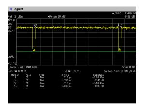
Duty Cycle = Ton / (Ton + Toff) =  $1392[\mu s] / (1392[\mu s] + 46[\mu s]) = 96.8[\%]$
