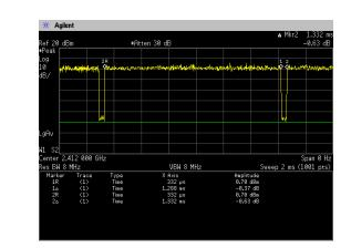
Duty Cycle = Ton / (Ton + Toff) =  $1288[\mu s] / (1288[\mu s] + 44[\mu s]) = 96.7[\%]$
