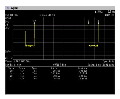
Duty Cycle = Ton / (Ton + Toff) =  $2124[\mu s]$  / ( $2124[\mu s]$  +  $376[\mu s]$ ) = 84.96[%]
