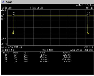
Duty Cycle = Ton / (Ton + Toff) =  $17020[\mu s] / (17020[\mu s] + 460[\mu s]) = 97.37[\%]$
