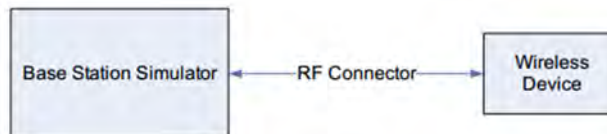
Figure 9.1 Power Measurement Setup
