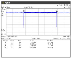
Duty Cycle = Ton / (Ton + Toff) =  $1023[\mu s] / (1023[\mu s] + 8[\mu s]) = 99.22[\%]$
