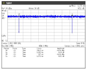
Duty Cycle =  $\frac{\text{Ton}}{(\text{Ton + Toff})} = \frac{1363[\mu \text{s}]}{(1363[\mu \text{s}] + 8[\mu \text{s}])} = 99.42[\%]$
