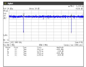
Duty Cycle =  $Ton / (Ton + Toff) = 1276[\mu s] / (1276[\mu s] + 8[\mu s]) = 99.38[%]$
