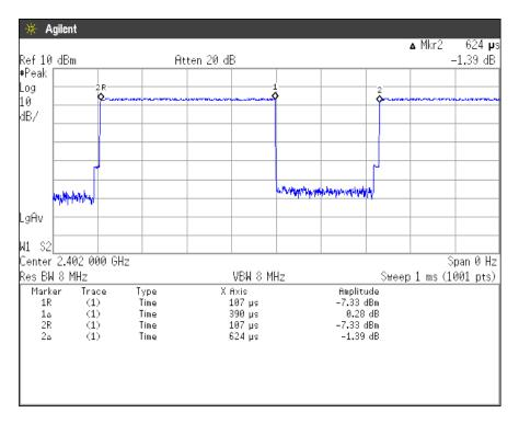
Duty Cycle = Ton / (Ton + Toff) =  $390[\mu s]$  / ( $390[\mu s]$  +  $234[\mu s]$ ) = 62.5[%]
