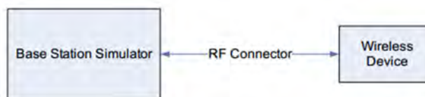
Figure 9.1 Power Measurement Setup
