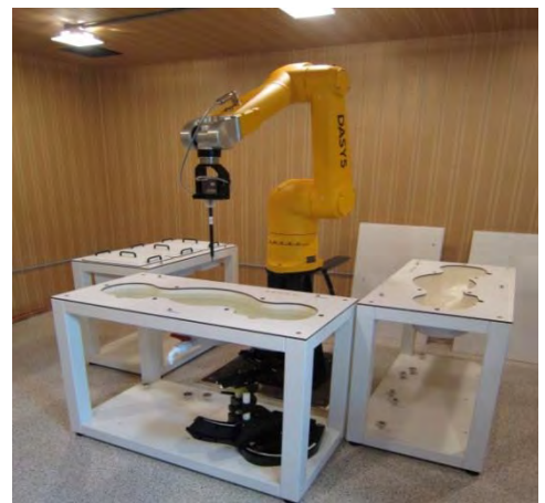
Figure E.7.1 DASY5 Test System
