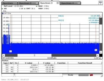
Aggregate Channel Closing Transmission Time S Dwell Ν Limit [points] [bins] [ms] [ms] [ms] [ms] 11200 11159 1.003674 0 0 60
