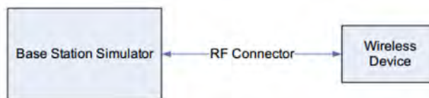
Figure 9.1 Power Measurement Setup
