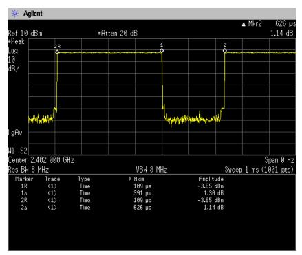
Duty Cycle = Ton / (Ton + Toff) =  $391[\mu s] / (391[\mu s] + 235[\mu s]) = 62.46[\%]$
