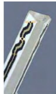
Figure E.2.2 Probe Thick-Film Technique
