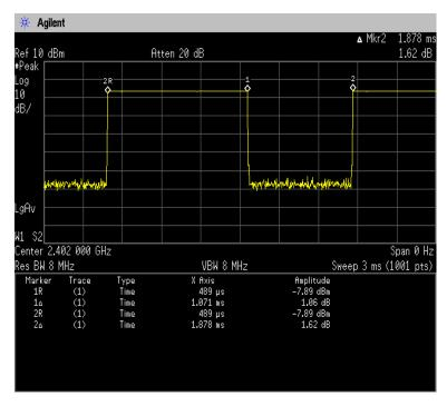
Duty Cycle = Ton / (Ton + Toff) =  $1071[\mu s] / (1071[\mu s] + 807[\mu s]) = 57.03[\%]$
