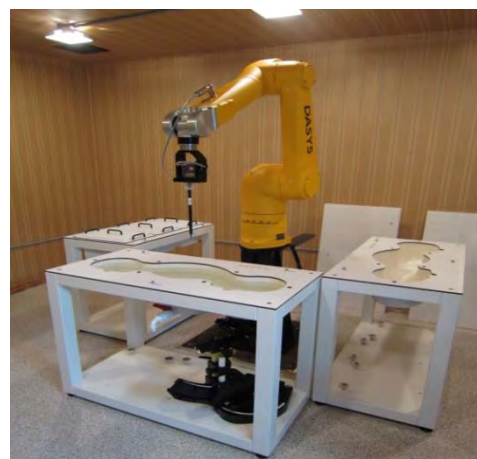
Figure E.7.1 DASY5 Test System
