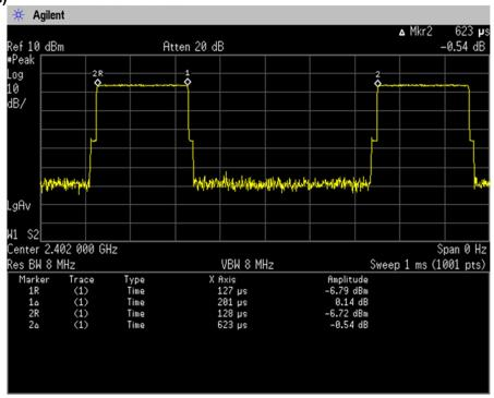
Duty Cycle = Ton / (Ton + Toff) =  $201[\mu s]$  / ( $201[\mu s]$  +  $422[\mu s]$ ) = 32.26[%]
