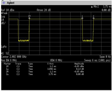
Duty Cycle = Ton / (Ton + Toff) =  $3096[\mu s]$  / ( $3096[\mu s]$  +  $654[\mu s]$ ) = 82.56[%]
