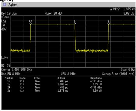
Duty Cycle = Ton / (Ton + Toff) =  $1065[\mu s] / (1065[\mu s] + 810[\mu s]) = 56.8[\%]$
