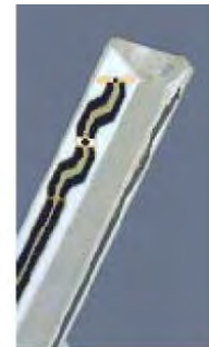
Figure E.2.2 Probe Thick-Film Technique
