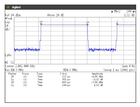
Duty Cycle = Ton / (Ton + Toff) =  $381[\mu s] / (381[\mu s] + 244[\mu s]) = 60.96[\%]$
