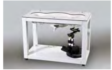
Figure E.5.1 SAM Twin Phantom
