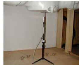
Figure 11.1 Dipole Verification Test Setup Diagram & Photo
