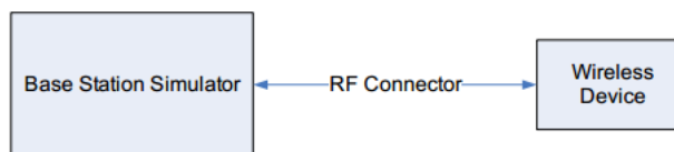
Figure 10.1 Power Measurement Setup
