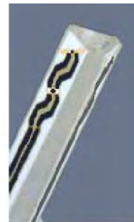
Figure E.2.2 Probe Thick-Film Technique
