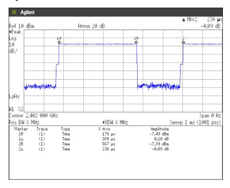
Duty Cycle = Ton / (Ton + Toff) =  $389[\mu s] / (389[\mu s] + 236[\mu s]) = 62.24[\%]$
