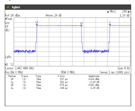
Duty Cycle = Ton / (Ton + Toff) =  $381[\mu s] / (381[\mu s] + 244[\mu s]) = 60.96[\%]$
