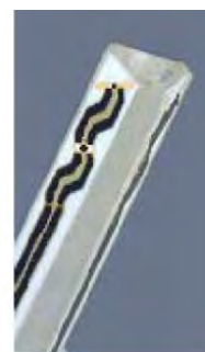
Figure E.2.2 Probe Thick-Film Technique
