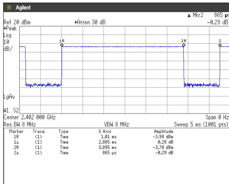
$$\text{Duty Cycle} = \text{Ton} / (\text{Ton} + \text{Toff}) = 2885[\mu\text{s}] / (2885[\mu\text{s}] + 865[\mu\text{s}]) = 76.93[\%]$$
