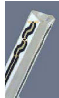
Figure 3.3 Probe Thick-Film Technique
