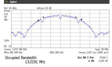
Transmit Freq Error -123.847 kHz x dB Bandwidth 8.544 MHz
