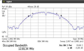
Transmit Freq Error -362.858 kHz x dB Bandwidth 8.082 MHz
