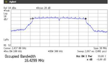
Transmit Freq Error -35.931 kHz x dB Bandwidth 15.744 MHz
