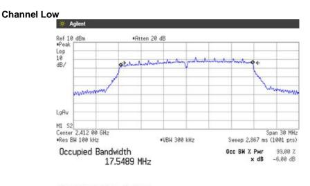
Transmit Freq Error 81.401 kHz x dB Bandwidth 16.332 MHz
