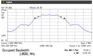
Transmit Freq Error 3.188 kHz x dB Bandwidth 677.415 kHz
