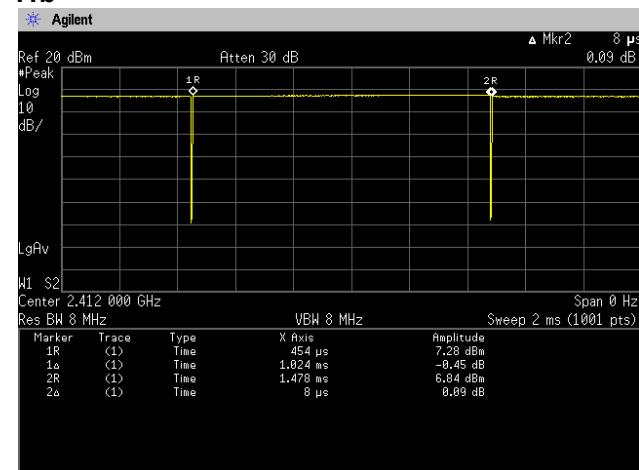
$$\text{Duty Cycle} = \text{Ton} / (\text{Ton} + \text{Toff}) = 1024[\mu\text{s}] / (1024[\mu\text{s}] + 8[\mu\text{s}]) = 99.22\%$$
