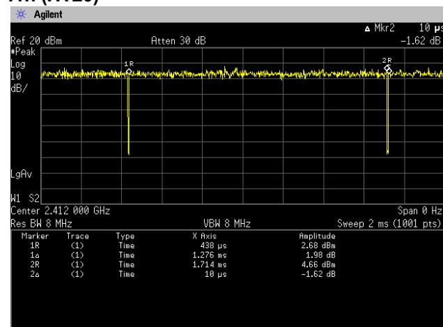
Duty Cycle = Ton / (Ton + Toff) = 1276[μs] / (1276[μs] + 10[μs]) = 99.22[%]
