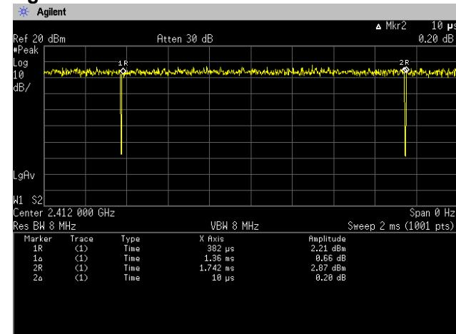
$$\text{Duty Cycle} = \text{Ton} / (\text{Ton} + \text{Toff}) = 1360[\mu\text{s}] / (1360[\mu\text{s}] + 10[\mu\text{s}]) = 99.27\%$$
