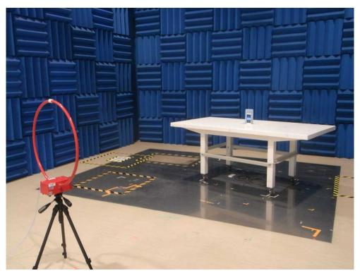
Radiated Emission for 30MHz to 300MHz
