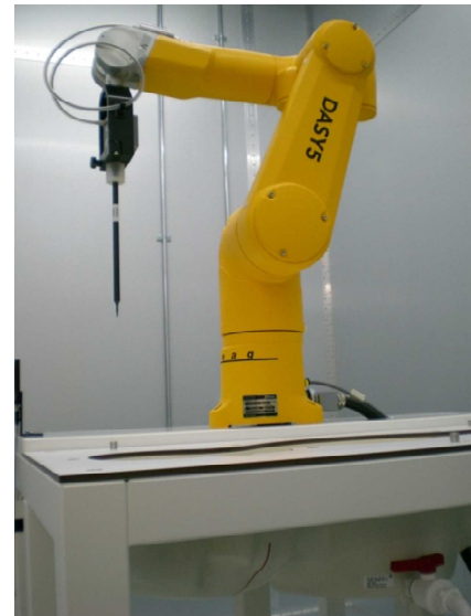
Figure 5.1 DASY5 Test System
