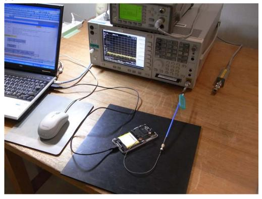
Transmitter Radiated Spurious Emissions (RF Radiated test)
