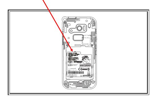
The label is attached to this device by an adhesive. The adhesive is permanent type with strong strength. Additionally, the label is readily to the purchaser at the time of purchase.
