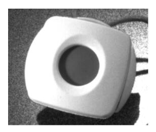
The Dual Tech Pendant (DTP) is an emergency device which is intended to be carried by persons under risk. It is activated by a momentarily button depression. Once activated it sends a FM signal which lasts for 2 seconds which will be received by the nearest base station receiver in the area. The modulation signal is a data stream having the base-band frequency in the range of 500-700Hz.
