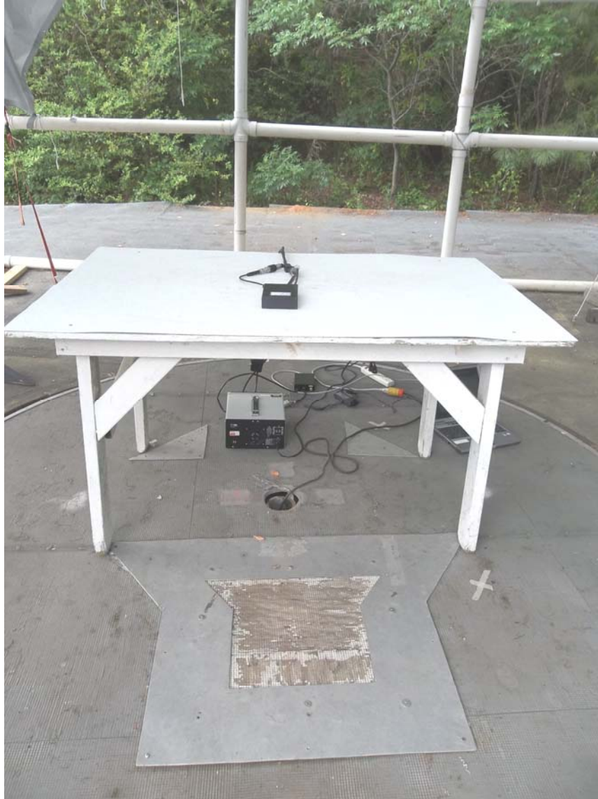
Figure 1- Radiated Emissions Test Setup (Front)
