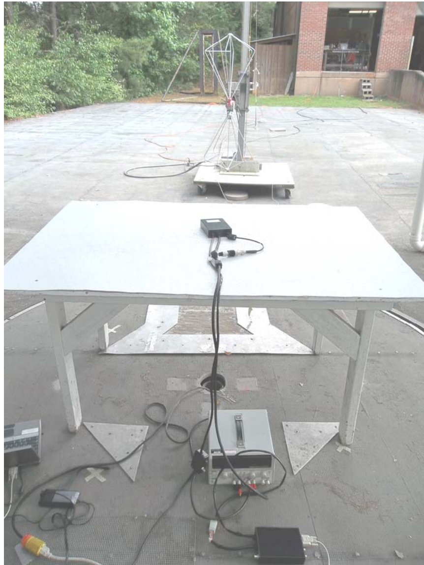
Figure 2. Radiated Emissions Test Setup (Rear 30-200 MHz)
