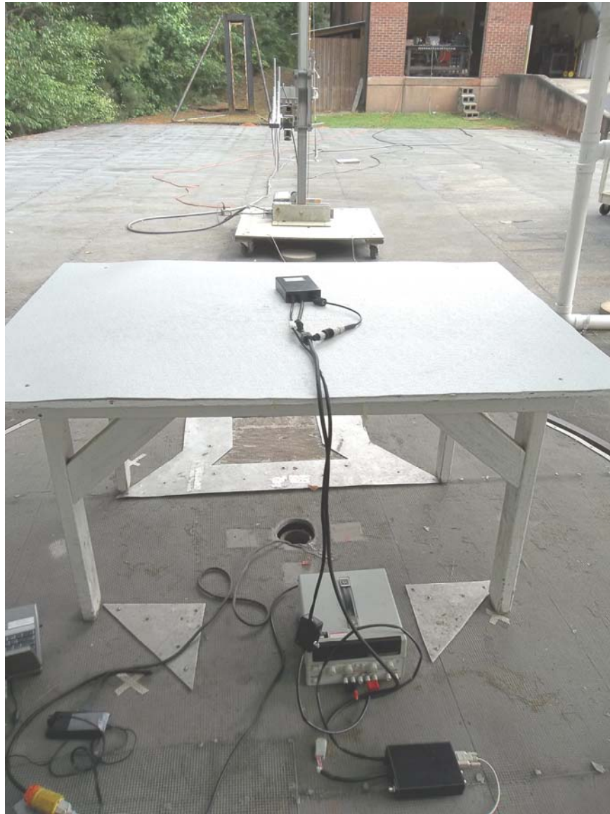
Figure 3. Radiated Emissions Test Setup (Rear 200 -1000 MHz)
