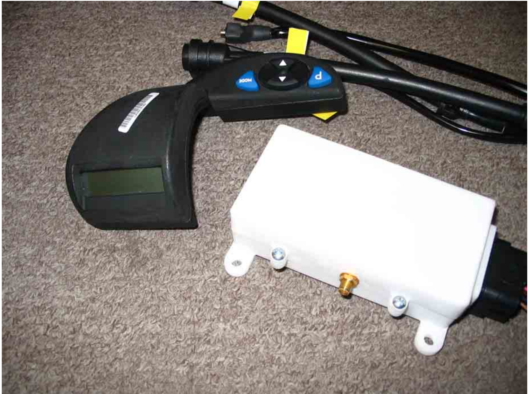
Figure 2: GMSH with Handlebar Controls
