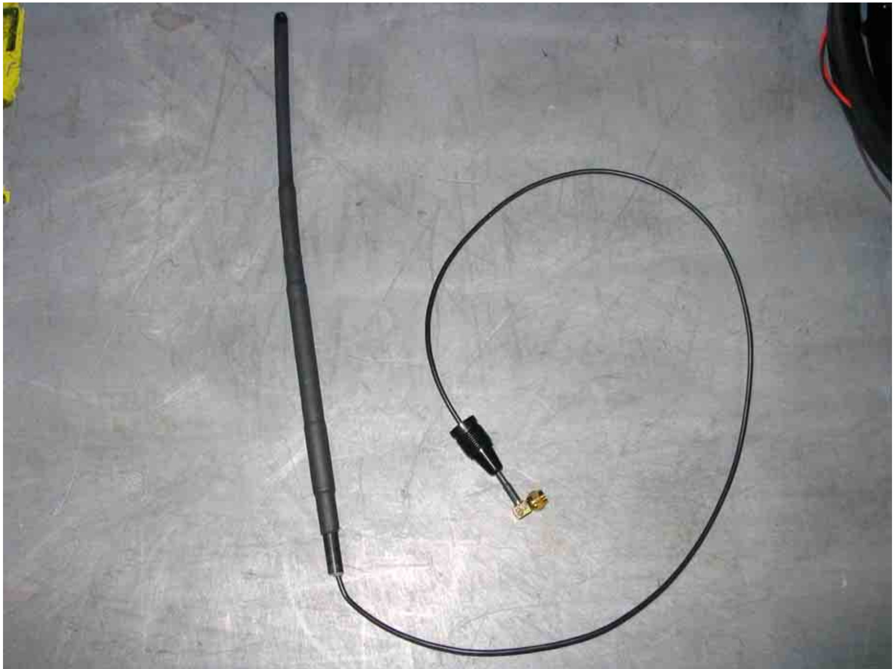
Figure 5: Sleeve Dipole Antenna with Connecting Cable
