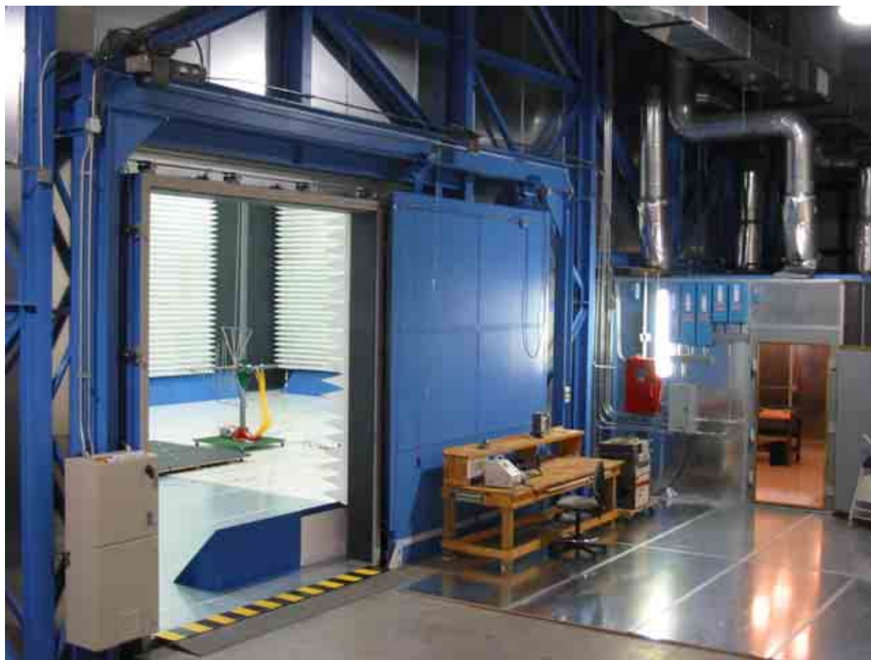
Figure 3-1: 10-Meter EMC Site
