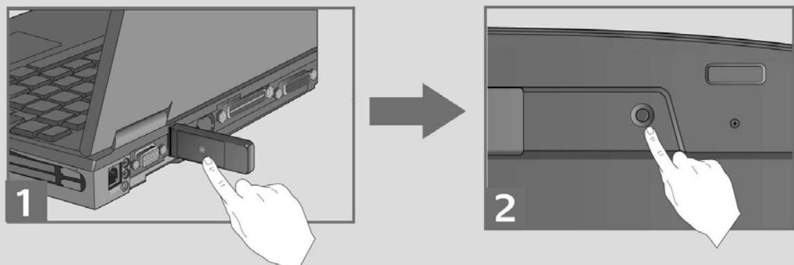
**English Solving Setup Problems.** 1. Check cable connection. 2. Place receiver in USB stand away from electrical devices; avoid metallic surfaces. 3. Check battery installation. 4. Turn **ON** mouse by pressing Power button for 2 seconds. Mouse is ON when LED is ON. **5. Establish connection:** 1) Press red Connect button under the receiver, and then 2) **QUICKLY** press red Connect button under device.
