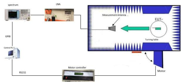
Block diagram to show the chamber and test equipment.
