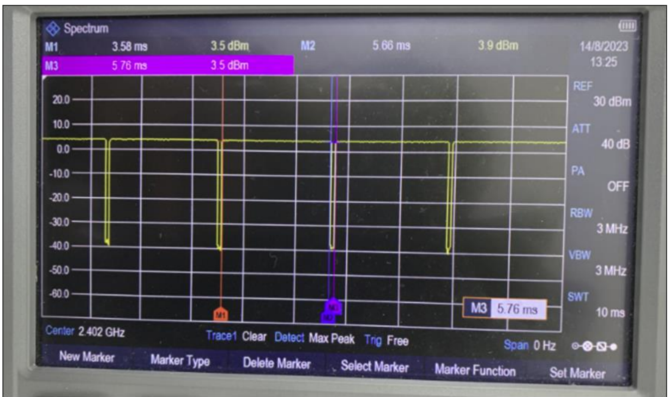
Time-domain plot for Bluetooth transmission signal
